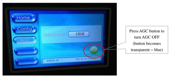
2. Adjust the Exciter POWER setting under the RF submenu to achieve the desired Forward System Power (1000W for example) as monitored on the Controller Home screen.
