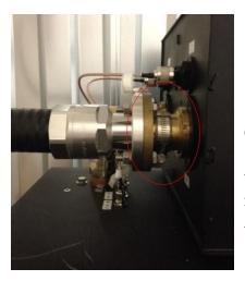
(<u>Please note</u>: If your Antenna feed is other than 1 5/8 EIA flanged (as shown on left), then you will need to provide whatever adapter hardware is necessary to facilitate this connection to your Antenna feed).
