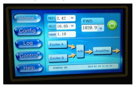
The home screen is divided into 4 parts: Title Bar (left column), Power Metering (upper right), Block Diagram (middle right) and Status Bar (lower right), as shown below.
