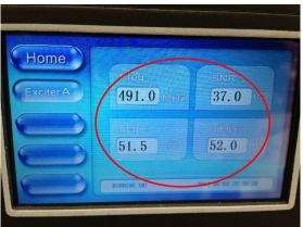
8. With your TX operating at your desired output power and with good RF performance, the next step is to set up and re-engage the TX AGC. To accomplish this, slowly increase the value of POWER in the Exciter RF submenu to raise the output power of the system to 1.1 x desired TPO (for example 1100W if a 1000W TPO level is desired). (Note: You are bringing up the TX to 1.1 x desired TPO to provide 10% headroom for AGC operation).
