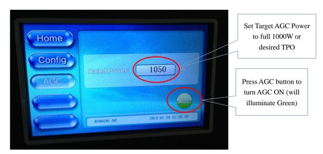
10. Press the HOME button to return to the HOME screen to monitor FWD power as it slowly reduces from 1.1 x TPO to the AGC target power (desired TPO) level over the next minute or so. With the AGC engaged, the FWD power metering may vary up to +/- 5%, so for a 1000W TX, meter variations from 950W to 1050W may be experienced.
