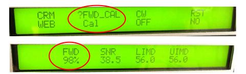
Please note that the Exciter FWD PWR meter reading is based on the RF\_IN\_A BNC feedback sample on the rear panel of the Exciter and is only available when this sample is connected and in the proper signal level range (40% < FSSIA < 75%).
