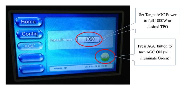
12. Press the HOME button to return to the HOME screen to monitor FWD power as it slowly reduces from 1.1 x TPO to the AGC target power (desired TPO) level over the next minute or so. With the AGC engaged, the FWD power metering may vary up to +/- 5%, so for a 1000W TX, meter variations from 950W to 1050W may be experienced.
