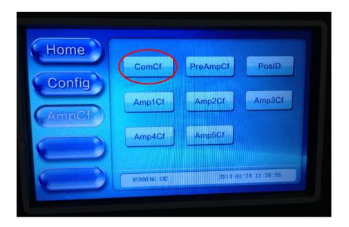
The ComCF screen is used to configure the TX maximum operating thresholds to engage safety and protective power reduction and shutdown mechanisms. Press the NextPage button to reach the FWD, REFL, and REJT power calibration screen below.
