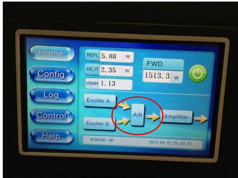
11. Your TX should now be up and running properly into your load or on-air antenna. Continue to monitor system parameters as you allow the transmitter to operate and stabilize at full output power for another 30 minutes.
