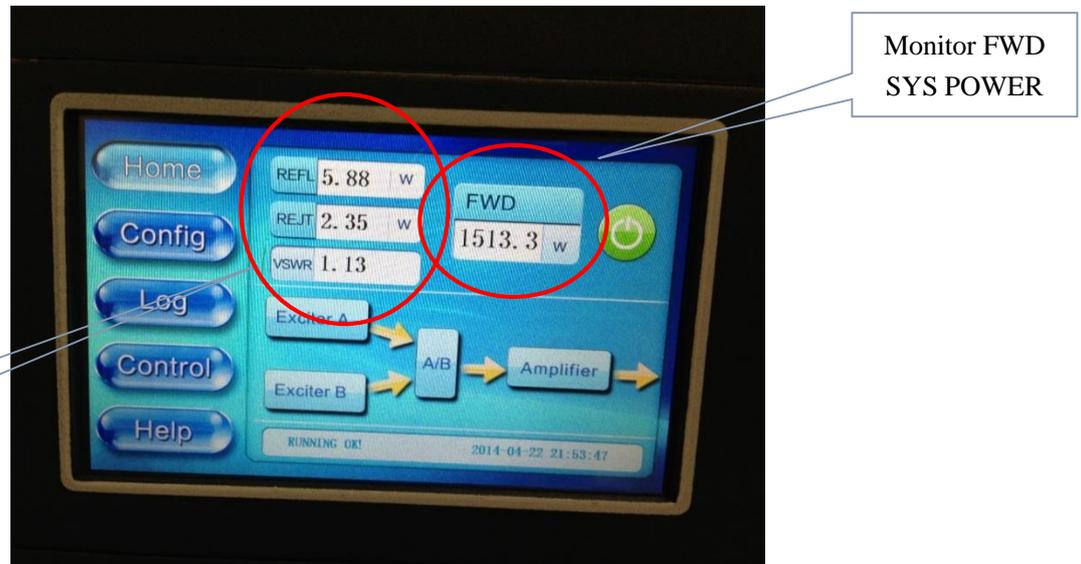
4. Slowly bring the FWD power to ~750W (half-power) and notice the power meter values of REFL, REJCT, and VSWR to be sure these look reasonable (less than a 1.5KW TX operating at a full 1500W FWD that has typical REFL, REJT, and VSWR as shown above).
