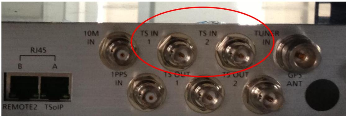
Please note: The above instructions apply to the 5X Exciter (which requires an ASI input signal) and is most likely the Exciter installed in your system. However, if you ordered the 9X Exciter (that can accept an ASI, SMPTE301M, or TSoIP (optional) TS input, the rear panel connections on your Exciter will look slightly different. Please consult your 9X User Manual for details.
