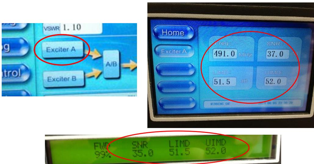
Linear and Non-Linear corrections were already performed and optimized at a TPO of 1500W in the factory and so the stored correction coefficients should produce good results.
