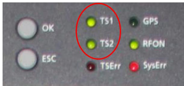
Please note: The Exciter SysErr LED illuminates solid RED when the Exciter is in Local mode and is OFF when the Exciter is in Remote mode. This LED only indicates a SysErr when flashing.
