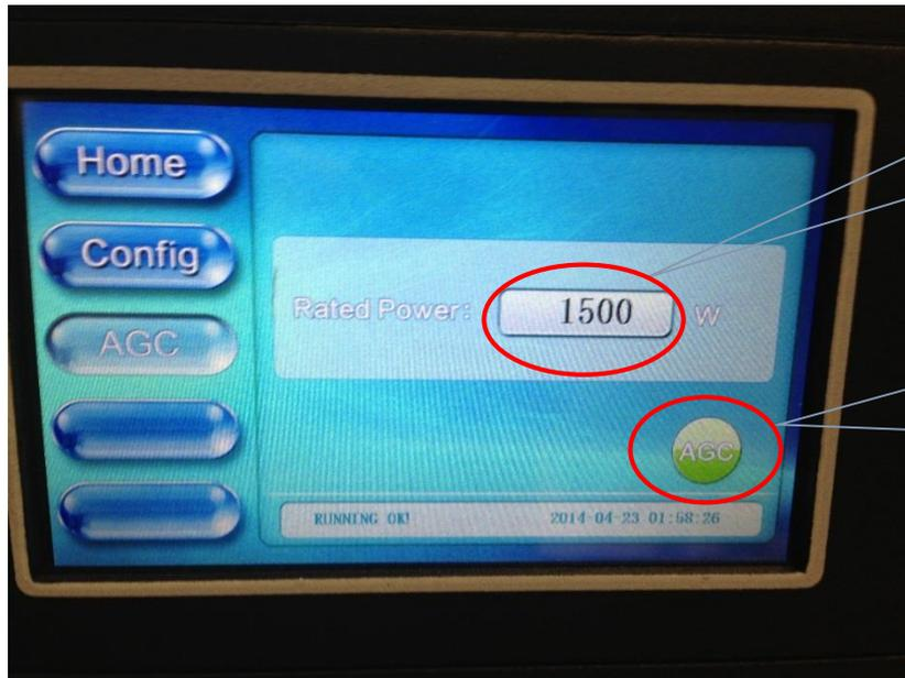
9. Press the HOME button to return to the HOME screen to monitor FWD power as it slowly reduces from 1.1 x TPO to the AGC target power (desired TPO) level over the next minute or so. With the AGC engaged, the FWD power metering may vary up to +/- 5%, so for a 1500W TX, meter variations from 1425W to 1575W may be experienced.
