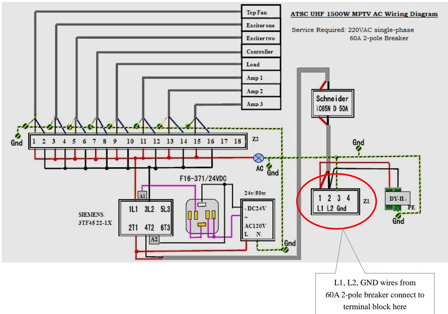
Properly connect the three wires to the terminal block as outlined in the above diagram, taking care to identify which terminal is connected to the chassis Ground in your system.
