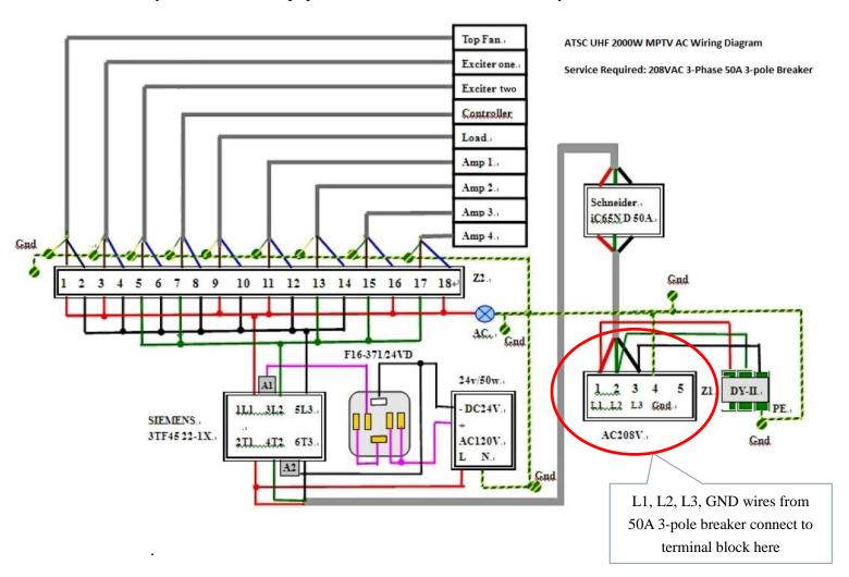
Properly connect the four wires to the terminal block as outlined in the above diagram, taking care to identify which terminal is connected to the chassis Ground in your system.
