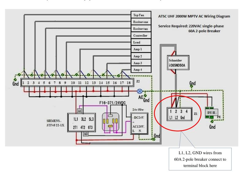
Properly connect the three wires to the terminal block as outlined in the above diagram, taking care to identify which terminal is connected to the chassis Ground in your system.
