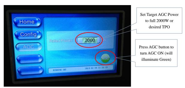
9. Press the HOME button to return to the HOME screen to monitor FWD power as it slowly reduces from 1.1 x TPO to the AGC target power (desired TPO) level over the next minute or so. With the AGC engaged, the FWD power metering may vary up to +/- 5%, so for a 2000W TX, meter variations from 1900W to 2100W may be experienced.
