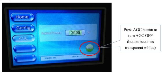
2. Adjust the Exciter POWER setting under the RF submenu to achieve the desired Forward System Power (2000W for example) as monitored on the Controller Home screen.
