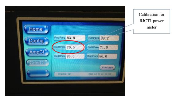
10. Repeat steps 3 through 7 above, this time removing, measuring, and returning the AUX IN sample to calibrate the Reject Load 2 system power meter by adjusting the value of Rejt2 below.
