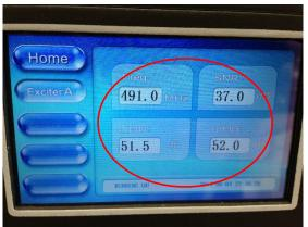
8. With your TX operating at your desired output power and with good RF performance, the next step is to set up and re-engage the TX AGC. To accomplish this, slowly increase the value of POWER in the Exciter RF submenu to raise the output power of the system to 1.1 x desired TPO (for example 2200W if a 2000W TPO level is desired). (Note: You are bringing up the TX to 1.1 x desired TPO to provide 10% headroom for AGC operation).
