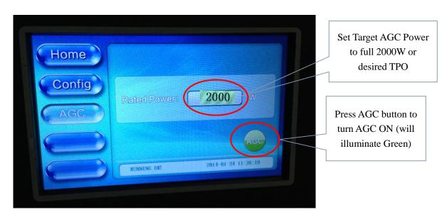
10. Press the HOME button to return to the HOME screen to monitor FWD power as it slowly reduces from 1.1 x TPO to the AGC target power (desired TPO) level over the next minute or so. With the AGC engaged, the FWD power metering may vary up to +/- 5%, so for a 2000W TX, meter variations from 1900W to 2100W may be experienced.
