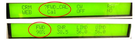
Please note that the Exciter FWD PWR meter reading is based on the RF\_IN\_A BNC feedback sample on the rear panel of the Exciter and is only available when this sample is connected and in the proper signal level range (40% < FSSIA < 75%).
