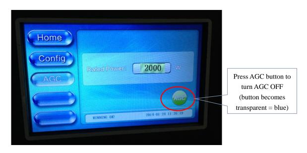
2. Adjust the Exciter POWER setting under the RF submenu to achieve the desired Forward System Power (2000W for example) as monitored on the Controller Home screen.
