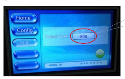
Set Target AGC to desired System Forward Power
