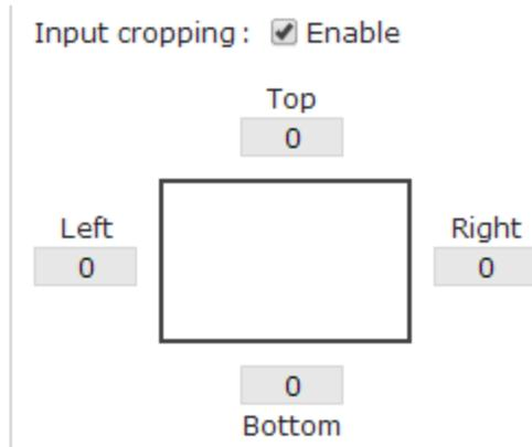
If cropping is used, it is recommended to crop to pixel boundary positions divisible by 16 to align on macroblock boundaries of the compressed video stream. This provides the best video quality during cropping.
