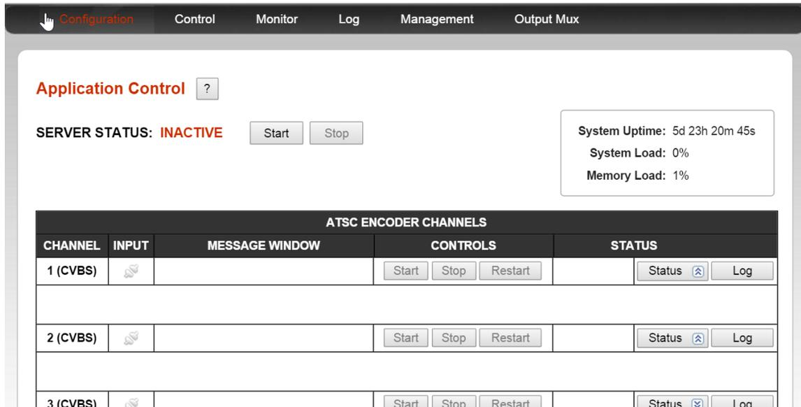
**SERVER STATUS:** This is a global ON/OFF control for the encoder. If the system is “INACTIVE” then select the Start button to change it to ACTIVE. The encoder will not run unless the SERVER STATUS is listed as ACTIVE.
