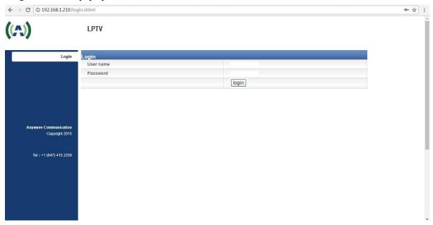
The "admin" tier provides full status and control of the PA and is accessed with a username and password of "anywavecom" and "anywavecom" (case sensitive).
