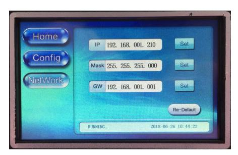
■ Set: There is a Set button for each bar in this screen. Pressing the Set button will lead to the corresponding configuration screen of IP or Mask or GateWay accordingly. Using the IP setting
