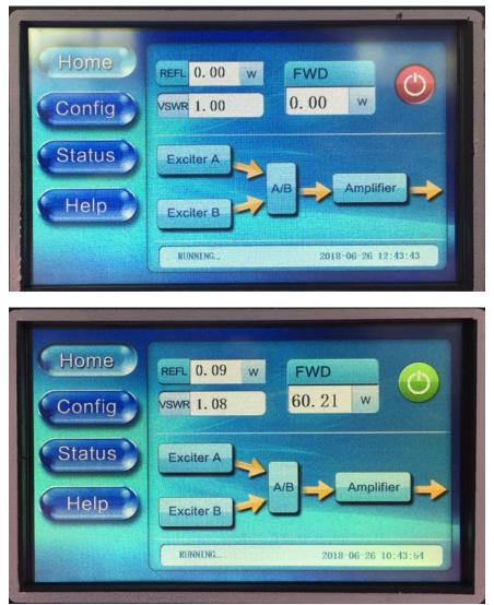
The home screen is divided into 4 parts: Title Bar (left column), Power Metering (upper right), Block Diagram (middle right) and Status Bar (lower right), as shown below.
