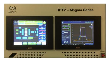
Innovative DDRF™ (Direct Digital RF) broadband automatic balancing technology achieves near perfect RF performance with shoulder levels exceeding -60 dB and out of band spurious also greater than -60 dB, all based on an ultra low noise floor.
