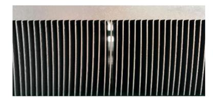
Oversized single-piece heat-sink provides even heat distribution and enhanced heat transfer
