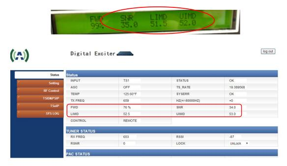
Linear and Non-Linear corrections were performed and optimized at the TX rated TPO in the factory and so the stored correction coefficients should produce good results if you are operating at or close to the TX max output power.
