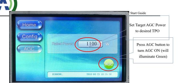
8. Press the HOME button to return to the HOME screen to monitor FWD power With the AGC engaged, the FWD power metering may vary up to +/- 5%, so for a 1500W TPO, meter variations from 1425W to 1575W may be experienced.
